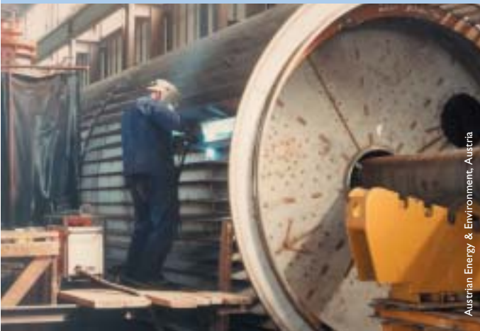
Dewatering-filter for the pulp industrie, base metal 1.4306 / AISI 304 L, welded with BÖHLER EAS 2-FD
