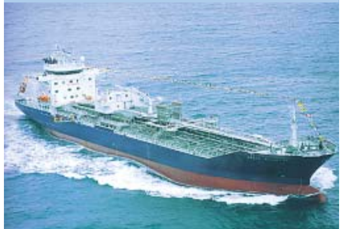
Chemical carrier, cargo vessels, UNS S 31803
