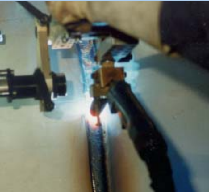
Mechanized welding with BÖHLER EAS 4 PW-FD
