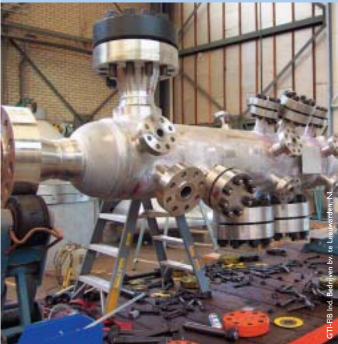
Apparatus construction: duplex steel UNS S31803 / 1.4462, wall thickness 30-40 mm, welded with BÖHLER CN 22/9 N-FD
