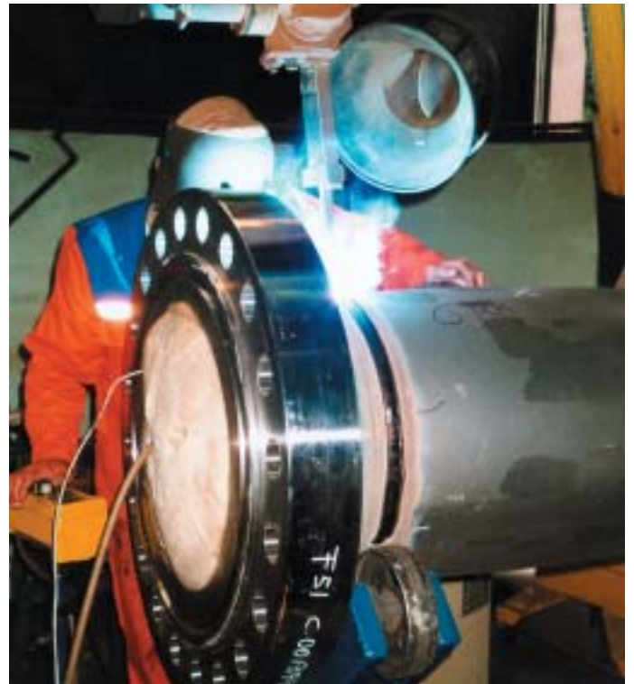
Pipe/flange joint weld made from duplex steel UNS S 31803 welded with BÖHLER CN 22/9 N-FD.
