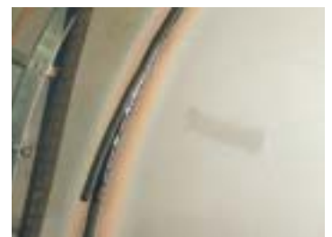
BÖHLER EAS 4 PW-FD with self-releasing slag and X-ray quality weld deposit.
