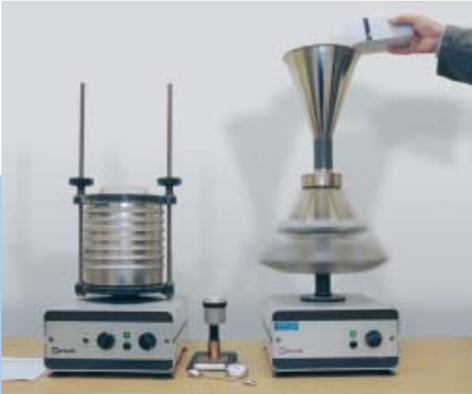
Screen analyses instrument to determine the powder grain size.
