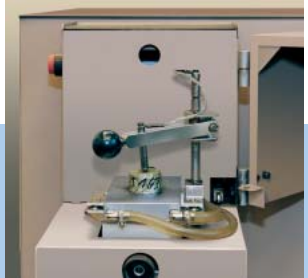
Optical emission spectrometer (OES) for the determination of the chemical analysis.
