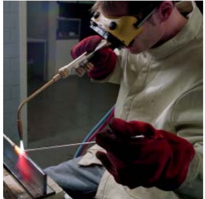
Gas welding with the casting rod BÖHLER Celsit V.
