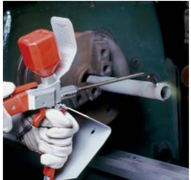
Flame spray welding with BÖHLER metal powder Niborit 4-P.
