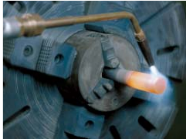
Flame spraying with BÖHLER metal powder Niborit 6-P.
