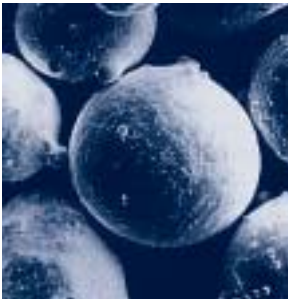
View through a scanning electron microscope of gas atomized spherical metal powder grains.
