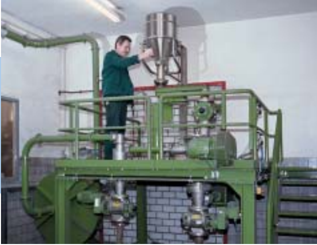
Wind screening for the powder grain size.
