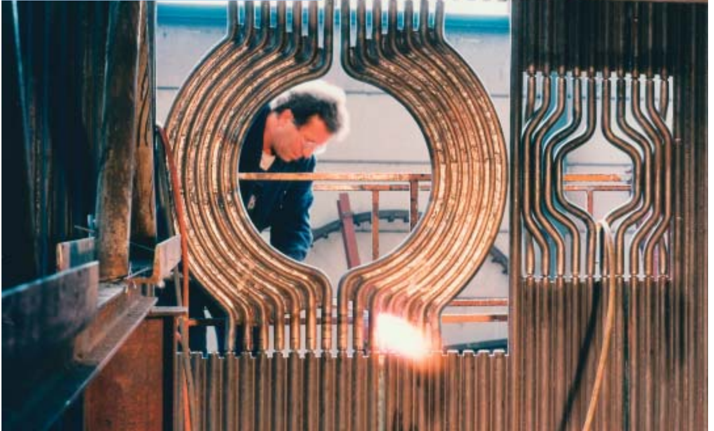
Segment of a boiler with circulating fluidized bed combustion.
